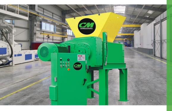
The CM Chip Shredder provides solutions for high volume production of specifically sized tire chips.
