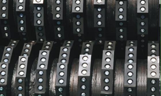
CM "Multi-Stack™" replaceable knife inserts are constructed with through hardened tool steel. These knives can be sharpened and reused up to 3 times.
